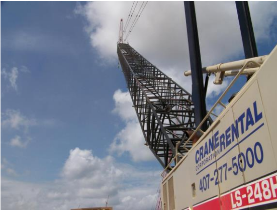
Picture of boom in the air 200feet of main and 50 feet of jib.
