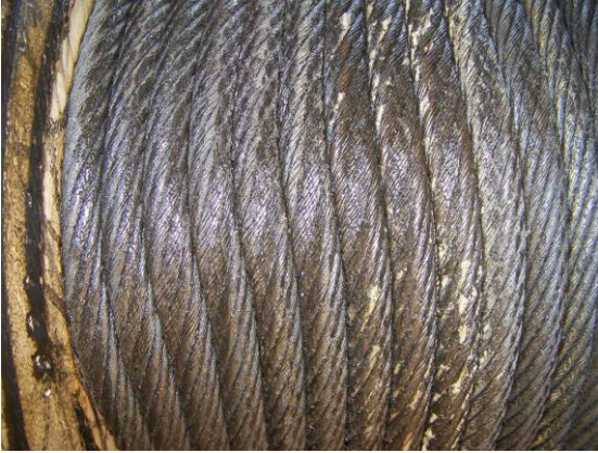
Picture of boom hoist cable crushing.
