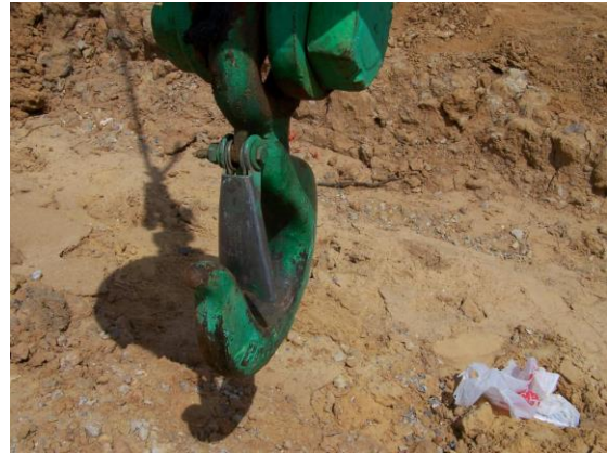
Picture of safety latch is bent to one side and should be replaced with a correct safety latch.
