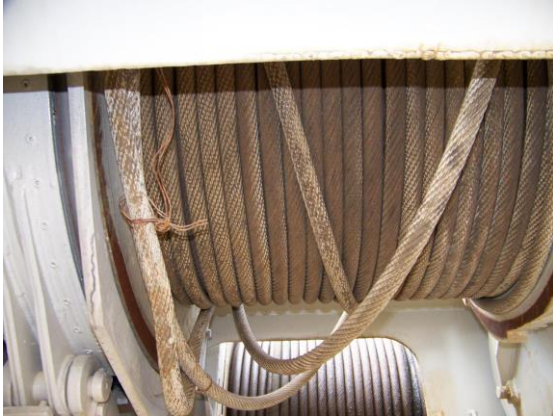
Picture of main hoist (rear drum) that is not being used and the rusted up condition of the cable.
