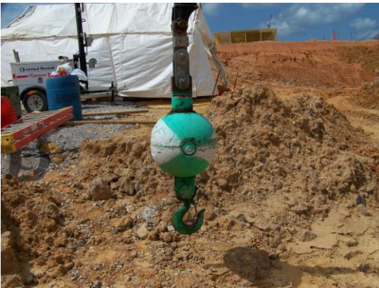
Picture of homemade weldment that is retaining the thru bolt.
