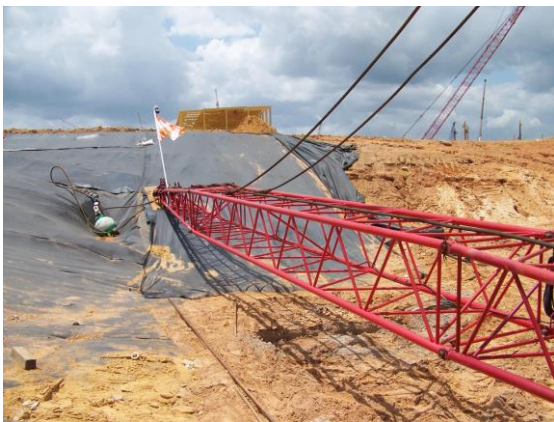
Picture of 1st section of jib past the Butt. 28M0916 S/N-L049208
