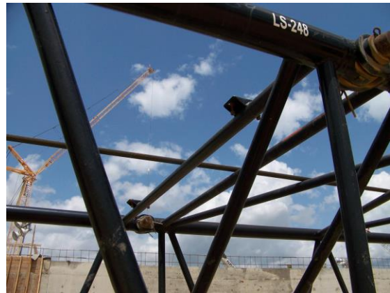
Picture of missing cable guide rollers on top of the boom.
