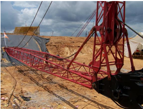
Picture of jib butt section. 28M0998 S/N-L049358
