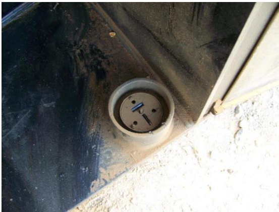
Picture of bubble level on the lower front frame that is unreadable.
