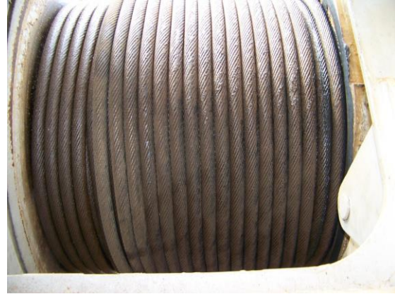
Picture of Au. Hoist (front drum) cable that needs to be lubricated.
