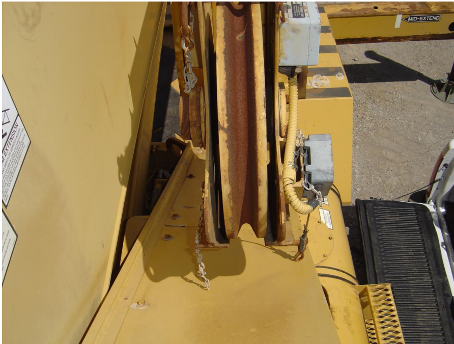
Picture of cable retaining pin that is missing from the tip of the jib.
