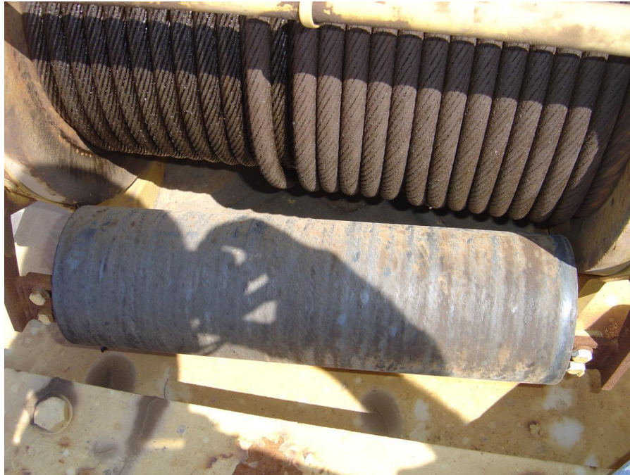
Picture of cable follower that is not working (froze up)
