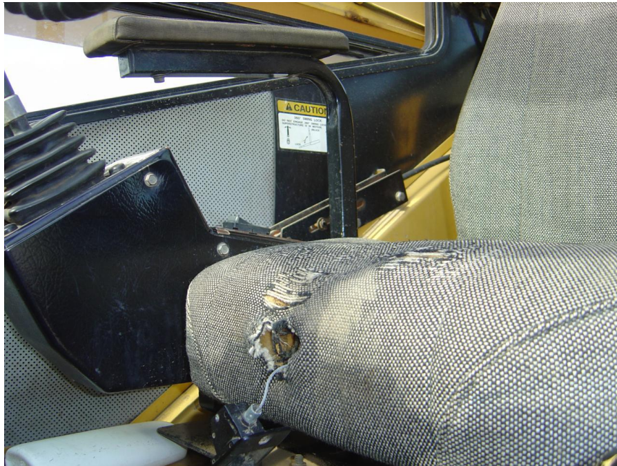
Picture of cable that is pulled out from the front of the seat, this cable works the back rest forwards or backwards.
