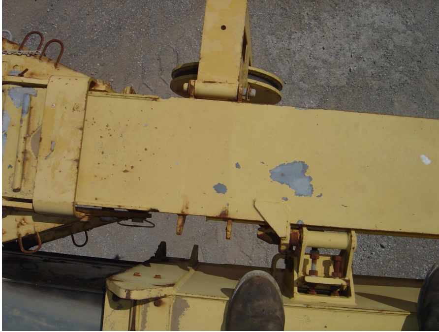
Picture of pin missing from rooster sheave on the jib.
