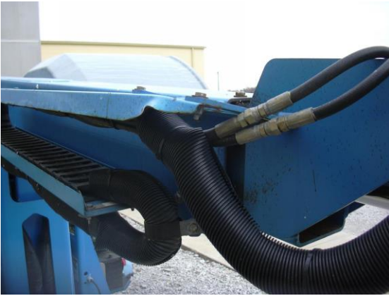
Picture of cable track that has been hit and bent up, that needs to be straightened.
